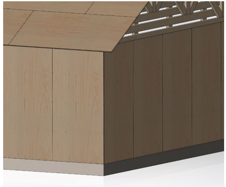
Fig. 13: Installation of plywood panels on a wall structure.
